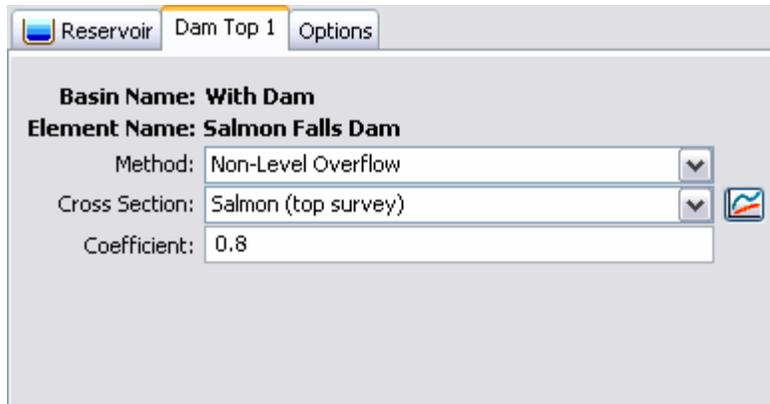
Figure 134. Dam top editor with the non-level overflow method selected.
