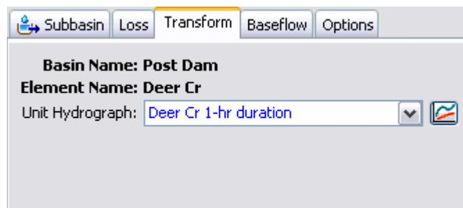
Figure 111. User-specified unit hydrograph transform method editor.
