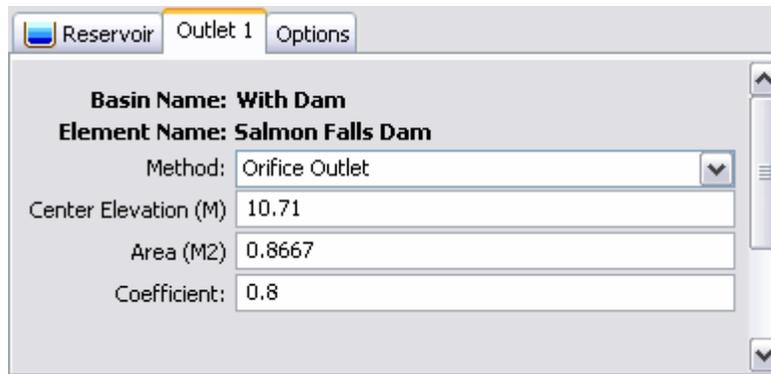
Figure 130. Outlet editor with the orifice method selected.
