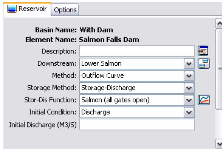
Figure 127. Reservoir component editor using the outflow curve method with a storage-discharge function.
